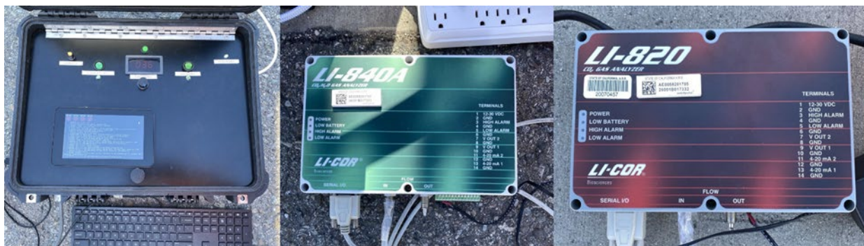
Figure 3. Receptors: (a) PEAQS, (b) LI-840A CO 2 Analyzer, and (c) LI-820 CO 2 Analyzer.
