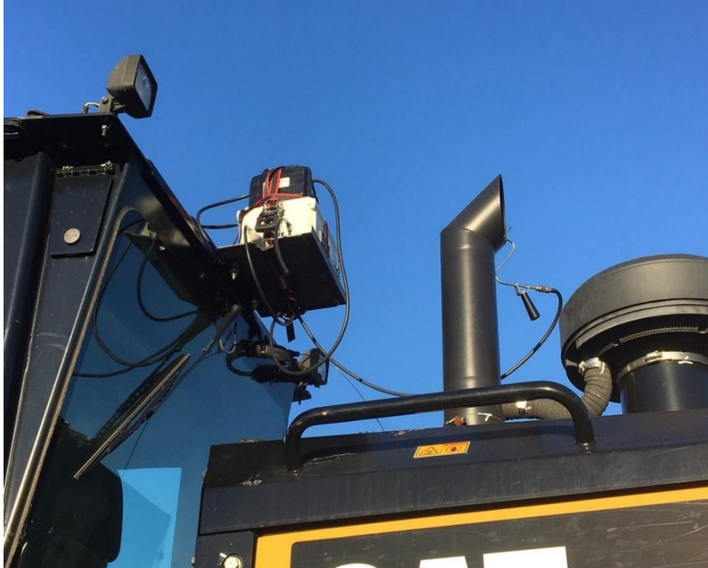
Figure 2: parSYNC Installed on Motor Grader
