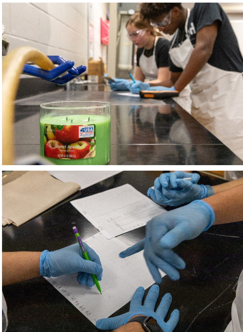
Figure 6. (Top panel) Students take PM_{10} measurements at directed time and distance intervals after extinguishing a candle. (Bottom panel) Students work in teams to translate data into a graph of PM_{10} concentrations over time.
