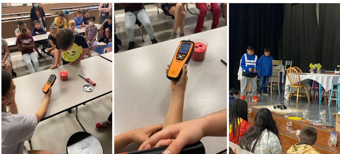
Figure 7. (Left panel) Students measure PM levels near a lit candle. (Middle panel) Students recognize an increase in PM levels after the candle is extinguished. (Right panel) Volunteers drive the remote-controlled car over the flour patch as they visualize tires kicking up particles.
